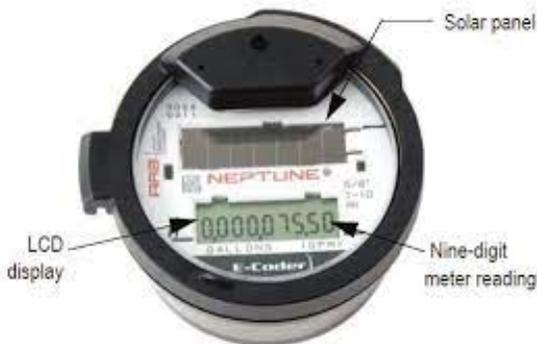
When the LCD displays the reading it will have seven numbers before the decimal point and two after. The numbers before the decimal point are whole numbers and after the decimal point are the fractions of a gallon. For example the reading below is Thirty-three thousand, Eighty -nine and a quarter of a gallon. We only read a thousand and above, so the reading would be 33.
